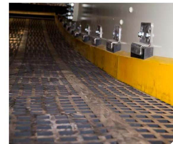
PU sideliners with chamfer top for Metso Outotec MF, mining screens
