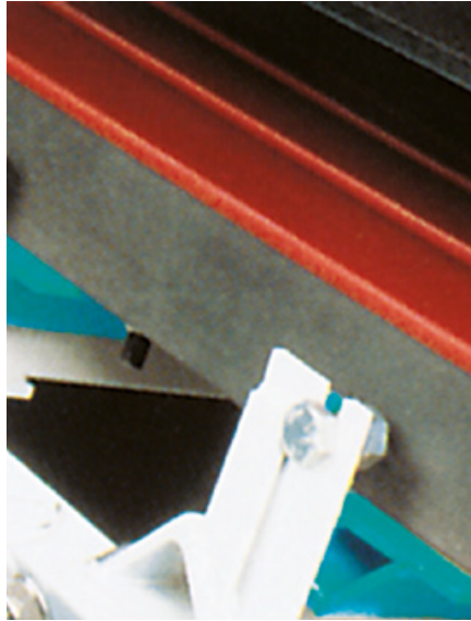
An adapter allows existing idler support to be used.
